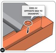
LOCATE A CLOSED GROMMET INTO THE ROOF GUTTER ON THE OPPOSITE SIDE TO THE DRAINPIPE LOCATION.
