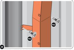
SECURE DRAINPIPE AT x6 LOCATIONS INDICATED USING TYPICAL FIXING METHOD. PLEASE NOTE: THE FIXING USED IS A SELF DRILLING COMPONENT.
