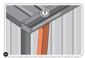
ALIGN DRAINPIPE 0205-51 WITH OPEN GROMMET WITHIN ROOF GUTTER.  $\underline{\textbf{IMPORTANT}}: \text{DRAINPIPE BRACKET IS LOCATED WITHIN SIDE PANEL RECESS}.$
