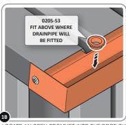
LOCATE AN OPEN GROMMET INTO THE ROOF GUTTER ABOVE WHERE THE DRAINPIPE WILL BE LOCATED.
