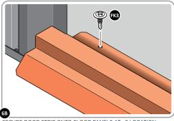
SECURE DOOR STRIP ONTO FLOOR PANELS AT  $\times 6$  LOCATION INDICATED.
