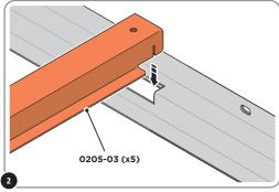
SLOT EACH FLOOR BRACE 0205-03 INTO POSITION AS SHOWN ABOVE.
