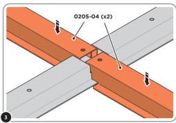
SLOT EACH FLOOR BRACE 0205-04 INTO POSITION AS SHOWN ABOVE. PLEASE NOTE: ENSURE TOP OF FLOOR BRACE IS LEVEL WITH TOP OF FLOOR RAIL.
