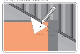
USE TEMPLATE BELOW TO MARK OUT SUGGESTED LOCATIONS FOR SECURING FLOOR TO BASE.
