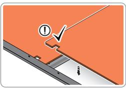
LOCATE EACH FLOOR PANEL 0204-32 OR 0204-69 INTO BASE OF STORAGE UNIT AS SHOWN.
