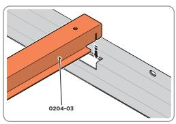
SLOT EACH FLOOR BRACE 0204-03 INTO POSITION AS SHOWN ABOVE.
