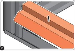
REMOVE DOOR STRIP 0204-71 FROM FLOOR PANELS AS SHOWN.
