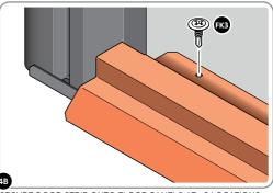
SECURE DOOR STRIP ONTO FLOOR PANELS AT x6 LOCATIONS INDICATED.
