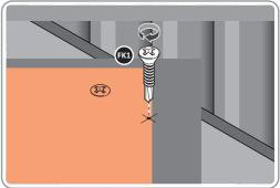
USE DRILL TO SECURE FIXING SCREW FK1 TO EACH FLOOR PANEL MARKED.
