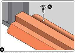
SECURE DOOR STRIP ONTO FLOOR PANELS AT X6 LOCATION INDICATED.
