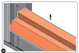
REMOVE DOOR STRIP 0205-74 FROM FLOOR PANELS AS SHOWN.
