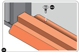
SECURE DOOR STRIP ONTO FLOOR PANELS AT x6 LOCATION INDICATED. PLEASE NOTE: THE FIXING USED IS A SELF DRILLING COMPONENT.
