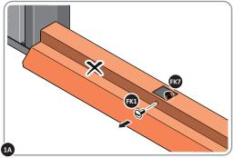
REMOVE NUT AND BOLT FROM DOOR STRIP AT x2 LOCATIONS INDICATED.
