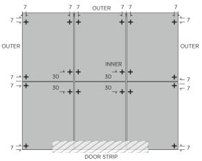
ASSEMBLY STAGE 7B LOCATE FIXING SCREW AND DRILL TO FLOOR
