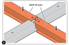
SLOT EACH FLOOR BRACE 0213-10 INTO POSITION AS SHOWN ABOVE. PLEASE NOTE: ENSURE TOP OF FLOOR BRACE IS LEVEL WITH TOP OF FLOOR RAIL
