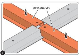
SLOT EACH FLOOR BRACE 0215-08 INTO POSITION AS SHOWN ABOVE. PLEASE NOTE: ENSURE TOP OF FLOOR BRACE IS LEVEL WITH TOP OF FLOOR RAIL
