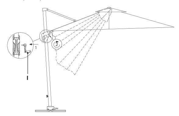
To adjust the angle of the parasol, squeeze the handle then slide it to the hole position that gives the parasol the desired angle. Release the handle to lock.
