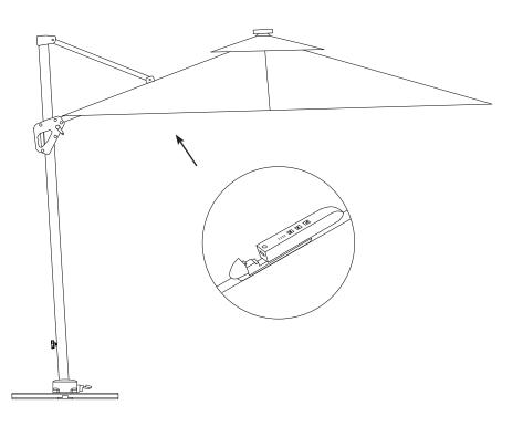
To rotate push down on the foot pedal then turn the parasol from the upright.
