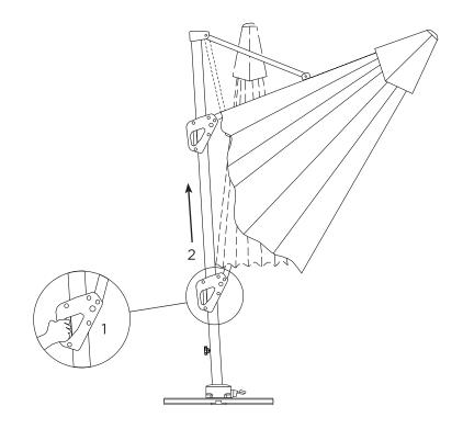
Insert the winder and rotate clockwise to open the parasol.
