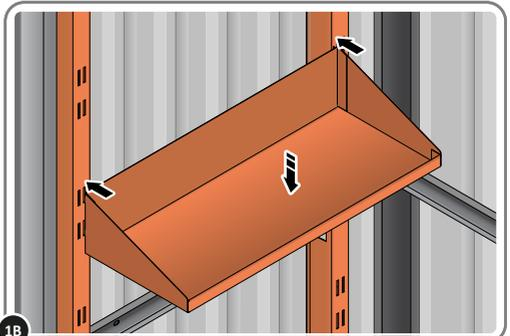
**1B** LOCATE EACH SHELF 0203-38-02 ONTO SHELF POST AS DESIRED. PLEASE NOTE: THE SHELF SIMPLY HOOKS ONTO THE POST.
