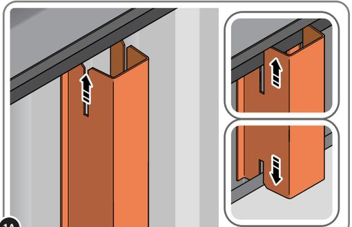
**1A** SLIDE SHELF POST UP INTO ROOF FRAME, ONCE THERE IS ENOUGH CLEARANCE AT THE BOTTOM LOCATE SHELF POST OVER FLOOR FRAME AND LOWER.
