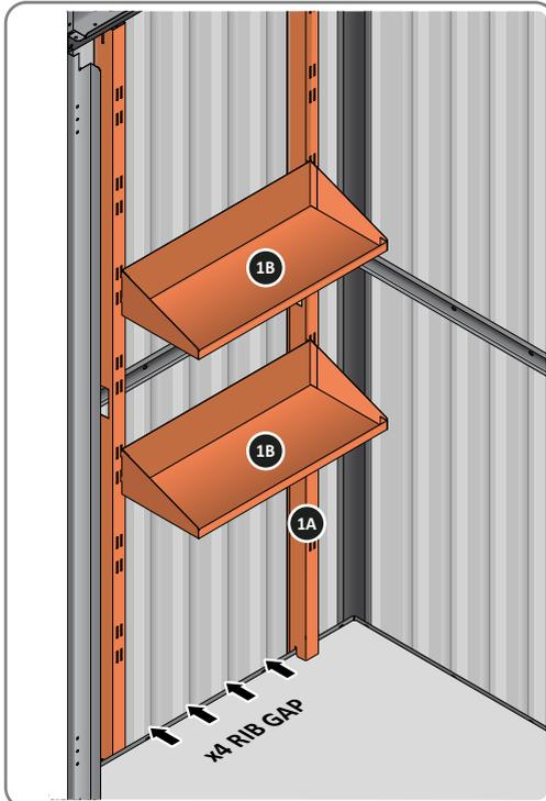
THE SHELF ASSEMBLY CAN BE LOCATED AS DESIRED, PLEASE DETERMINE THE MOST SUITABLE LOCATION AND ASSEMBLE AS SHOWN IN FIG.1A & 1B.
