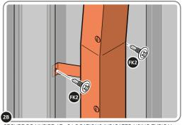
SECURE DRAINPIPE AT x6 LOCATIONS INDICATED USING TYPICAL FIXING METHOD.
