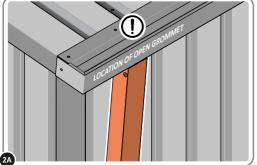
ALIGN DRAINPIPE 0205-51 WITH OPEN GROMMET WITHIN ROOF GUTTER. IMPORTANT: DRAINPIPE BRACKET IS LOCATED WITHIN SIDE PANEL RECESS.
