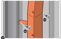
SECURE DRAINPIPE AT x6 LOCATIONS INDICATED USING TYPICAL FIXING METHOD. PLEASE NOTE: THE FIXING USED IS A SELF DRILLING COMPONENT.
