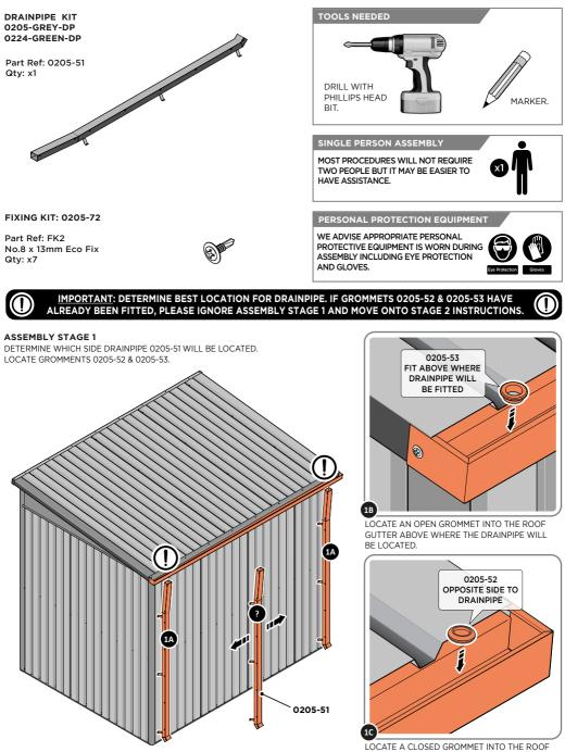
LOCATE A CLOSED GROMMET INTO THE ROO GUTTER ON THE OPPOSITE SIDE TO THE DRAINPIPE LOCATION. **Assembly Guide**
