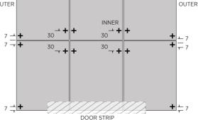
ASSEMBLY STAGE 7B LOCATE FIXING SCREW AND DRILL TO FLOOR
