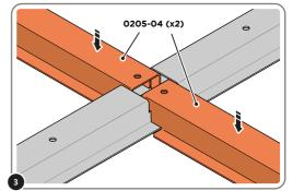
SLOT EACH FLOOR BRACE 0205-04 INTO POSITION AS SHOWN ABOVE. PLEASE NOTE: ENSURE TOP OF FLOOR BRACE IS LEVEL WITH TOP OF FLOOR RAIL.
