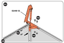
LOCATE LID AND SECURE RUBBER FEET & SPACERS. NOTE: USE A SCRATCH RESISTANCE SURFACE.
