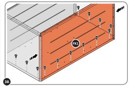
**NOTE:** INWARD ADJUSTMENT OF SIDE PANELS REQUIRED, SECURE ALL THREE PANELS TO BASE, AT LOCATIONS INDICATED ABOVE .
