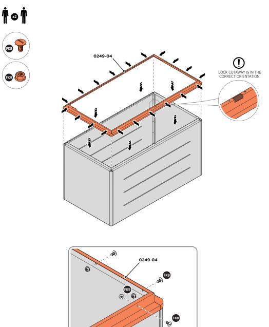
NOTE: MAKE SURE THE LOCK CUTAWAY IS IN THE CORRECT ORIENTATION. LOCATE AND SECURE FRAME 0249-04, AT LOCATIONS INDICATED ABOVE.
