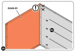
LOCATE AND LOOSELY ATTACH END PANELS TO BACK PANEL. IMPORTANT: ONLY ATTACH AT (x4) FIXING POINTS INDICATED AT THIS STAGE.
