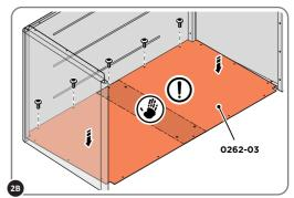
ONCE LOWERED INTO POSITION, LOOSELY ATTACH AT (x5) LOCATIONS. NOTE: IF APPLYING BODY WEIGHT TO FLOOR, ONLY USE AREA INDICATED ABOVE, WHICH HAS EXTRA STRENGTH AND SUPPORT.
