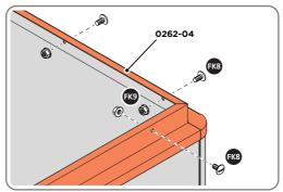
NOTE: MAKE SURE THE LOCK CUTAWAY IS IN THE CORRECT ORIENTATION. LOCATE AND SECURE FRAME 0262-04, AT LOCATIONS INDICATED ABOVE.
