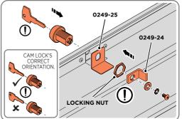
WITH THE LID IN THE UPSIDE DOWN POSITION, SECURE LOCK BACKING PLATE 0249-25 AND CAM LOCK ASSEMBLY TO LID AS SHOWN ABOVE. NOTE: M22 SOCKET WILL BE REQUIRED FOR LOCKING NUT.
