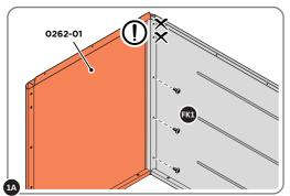
LOCATE AND LOOSELY ATTACH END PANELS TO BACK PANEL. IMPORTANT: ONLY ATTACH AT (x3) FIXING POINTS INDICATED AT THIS STAGE.
