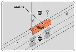
NOTE: MAKE SURE THE CATCH PLATE IS IN THE CORRECT ORIENTATION. LOCATE AND SECURE PLATE 0249-19, AT LOCATIONS INDICATED ABOVE.
