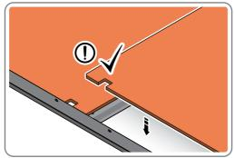
LOCATE EACH FLOOR PANEL 0204-32 OR 0204-69 INTO BASE OF STORAGE UNIT AS SHOWN.
