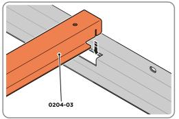
SLOT EACH FLOOR BRACE 0204-03 INTO POSITION AS SHOWN ABOVE.
