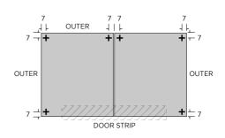
ASSEMBLY STAGE 5B LOCATE FIXING SCREW AND DRILL TO FLOOR
