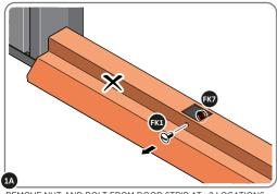
REMOVE NUT AND BOLT FROM DOOR STRIP AT x2 LOCATIONS INDICATED.
