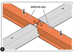
SLOT EACH FLOOR BRACE 0213-10 INTO POSITION AS SHOWN ABOVE. PLEASE NOTE: ENSURE TOP OF FLOOR BRACE IS LEVEL WITH TOP OF FLOOR RAIL
