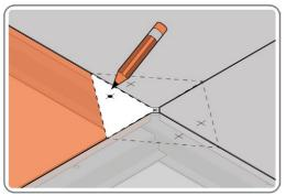
USE TEMPLATE BELOW TO MARK OUT SUGGESTED LOCATIONS FOR SECURING FLOOR TO BASE. (NOTE: ONLY MARK INNER CORNER PANELS - 7 x 30 mm).
