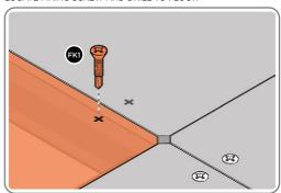
USE DRILL TO SECURE FIXING SCREW FK1 TO EACH FLOOR PANEL MARKED.
