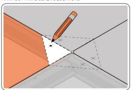
USE TEMPLATE BELOW TO MARK OUT SUGGESTED LOCATIONS FOR SECURING FLOOR TO BASE. (NOTE: ONLY MARK INNER CORNER PANELS -  $7\times30$  mm).
