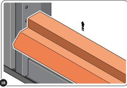
REMOVE DOOR STRIP 0205-74 FROM FLOOR PANELS AS SHOWN.
