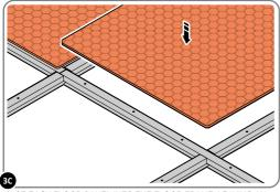
SLOT EACH FLOOR PANEL INTO THE FLOOR FRAME, LEAVING AN EQUAL SPACE BETWEEN EACH PANEL. AS SHOWN ABOVE.
