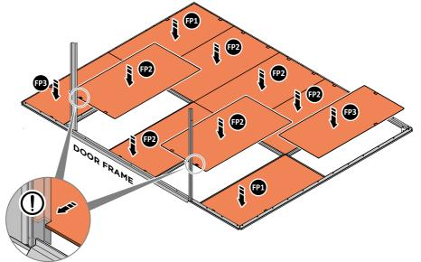
PANELS WILL REQUIRE REMOVAL OF CUT-OUT, CAREFULLY USING A HACKSAW
