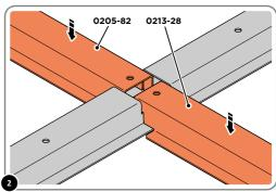
SLOT EACH FLOOR BRACE 0205-82 AND 0213-28 INTO POSITION. PLEASE NOTE: ENSURE TOP OF FLOOR BRACE IS LEVEL WITH TOP OF FLOOR RAIL, AS SHOWN ABOVE.
