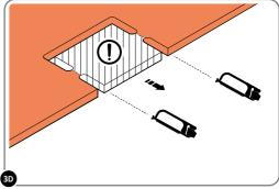
LOCATE FLOOR PANELS FP2 (x1) AND FP3 (x1). **NOTE**: REMOVE CUT-OUT ON OUTER SIDE, AND SLOT INTO DOOR FRAME. DESIGNED FOR EASY REMOVAL USING A HACKSAW.
