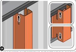
SLIDE SHELF POST UP INTO ROOF FRAME, ONCE THERE IS ENOUGH CLEARANCE AT THE BOTTOM LOCATE SHELF POST OVER FLOOR FRAME AND LOWER.
