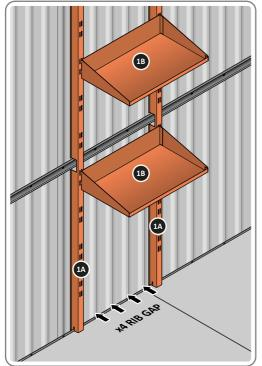
THE SHELF ASSEMBLY CAN BE LOCATED AS DESIRED, PLEASE DETERMINE LOCATE EACH SHELF 0205-38-02 ONTO SHELF POST AS DESIRED. THE MOST SUITABLE LOCATION AND ASSEMBLE AS SHOWN IN FIG.1A & 1B. PLEASE NOTE: THE SHELF SIMPLY HOOKS ONTO THE POST.
