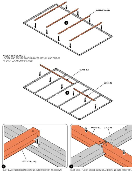
SLOT EACH FLOOR BRACE 0212-25 INTO POSITION AS SHOWN ABOVE.
