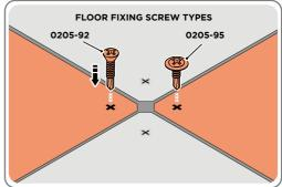
USE DRILL TO SECURE FIXING SCREW TO EACH FLOOR PANEL MARKED.
