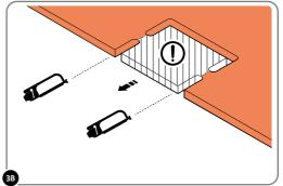
LOCATE FLOOR PANELS FP2 (x2). NOTE: REMOVE CUT-OUT ON OUTER SIDE, AND SLOT INTO DOOR FRAME. DESIGNED FOR EASY REMOVAL USING A HACKSAW.
