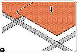
SLOT EACH FLOOR PANEL INTO THE FLOOR FRAME, LEAVING AN EQUAL SPACE BETWEEN EACH PANEL. AS SHOWN ABOVE. IMPORTANT: ENSURE FLOORING PATTERN IS FACING UPWARDS.
