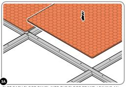
SLOT EACH FLOOR PANEL INTO THE FLOOR FRAME, LEAVING AN EQUAL SPACE BETWEEN EACH PANEL. AS SHOWN ABOVE. IMPORTANT: ENSURE FLOORING PATTERN IS FACING UPWARDS.
