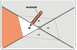
USE TEMPLATE BELOW TO MARK OUT SUGGESTED LOCATIONS FOR SECURING FLOOR TO BASE. 7 MM).
