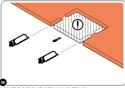
LOCATE FLOOR PANELS FP1 (x1) AND FP3 (x1). **NOTE**: REMOVE CUT-OUT ON OUTER SIDE, AND SLOT INTO DOOR FRAME. DESIGNED FOR EASY REMOVAL USING A HACKSAW.
