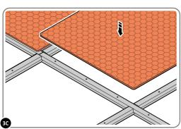
SLOT EACH FLOOR PANEL INTO THE FLOOR FRAME, LEAVING AN EQUAL SPACE BETWEEN EACH PANEL. AS SHOWN ABOVE.
