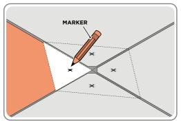
USE TEMPLATE BELOW TO MARK OUT SUGGESTED LOCATIONS FOR SECURING FLOOR TO BASE. 7 MM).
