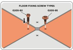
USE DRILL TO SECURE FIXING SCREW TO EACH FLOOR PANEL MARKED.
