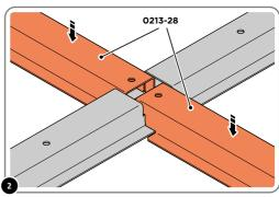
SLOT FLOOR BRACES 0213-28 INTO POSITION.
