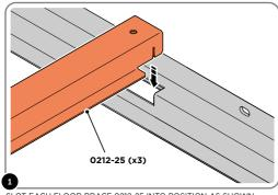
$\bar{\text{SLOT}}$  EACH FLOOR BRACE 0212-25 INTO POSITION AS SHOWN ABOVE.
