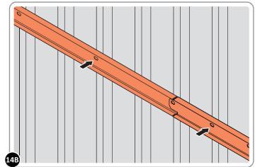
LOOSELY ATTACH CENTRE BRACE 0212-03 AT LOCATIONS INDICATED. SECURE SHORT CENTRE BRACE 0213-31 AT TWO LOCATIONS **IMPORTANT**: DO NOT SECURE AT OUTER FIXING POINT INDICATED.
