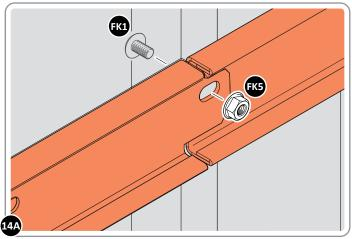
LOCATE AND LOOSELY ATTACH SHORT CENTRE BRACE 0213-31 AND CENTRE BRACE 0212-03 AS SHOWN AT LOCATIONS INDICATED ABOVE.
