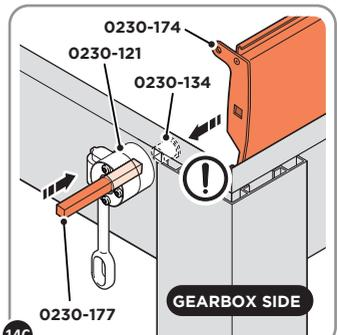
LOCATE AND PUSH DRIVING PIN 0230-177 THROUGH GEARBOX AND BUSH 0230-134, SECURE LOUVER 0230-174 TO DRIVING PIN.
