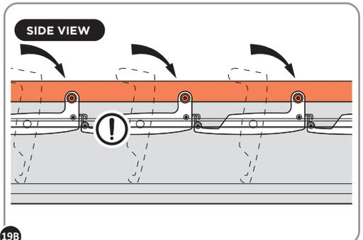
WITH THE LINK ARMS CONNECTED, ALLOW THE LOUVERS TO REST IN THEIR CLOSED POSITION.
