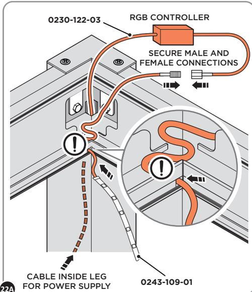
22A LOCATE RGB CONTROLLER 0230-122-03 AND CONNECT TO LED LIGHT CONNECTOR 0243-109-01. POSITION CABLE THROUGH GAP, AS SHOWN ABOVE.
