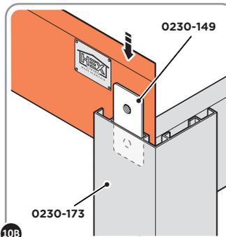
10B ENSURE FIXING PLATE 0230-149, SLOTS INTO TOP OF THE PERGOLA LEG, AS SHOWN ABOVE.
