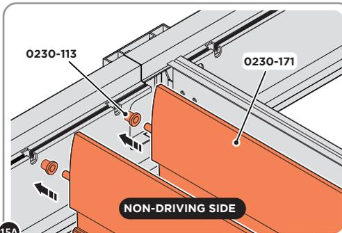
15A SECURE LOUVER BEARING 0230-113, ONTO HORIZONTAL BEAM 0243-111. INSERT LOUVER 0230-171 INTO BEARING, AS SHOWN ABOVE.
