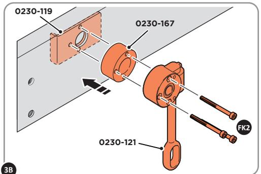
**3B** LOCATE AND SECURE GEARBOX 0230-121 & SPACER 0230-167 TO FIXING PLATE 0230-119, USING THREE BOLTS, AS SHOWN ABOVE.
