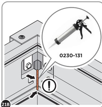
CORNER SECTIONS SHOULD BE MADE WATERTIGHT WITH SEALANT PROVIDED.
