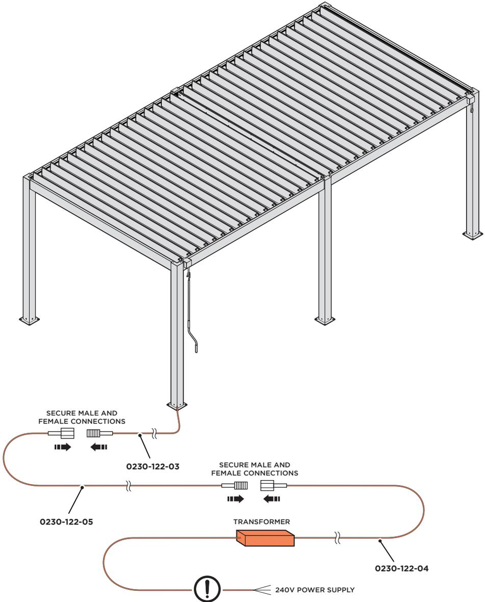
**IMPORTANT: USE A QUALIFIED ELECTRICIAN WHEN CONNECTING THE LED LIGHTING TO A MAINS SUPPLY.**
