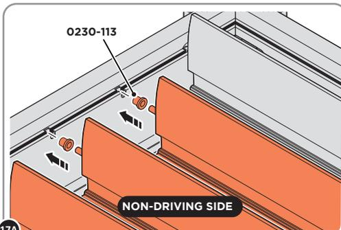
**17A** LOCATE AND SECURE LOUVER BEARING 0230-113 ONTO LOUVER 0230-104, SECURE TO BEAM 0243-110 ON NON-DRIVE SIDE.
