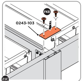
LOCATE CENTRE POST CAPS 0243-103 AND SECURE TO PERGOLA LEGS USING (X2) ECO FIX SCREWS (FK8).
