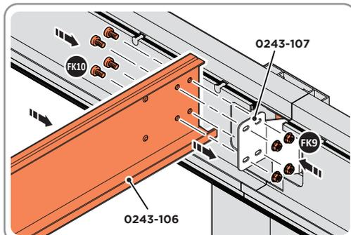
LOCATE CENTRAL BEAM 0243-106, FIT TO BEAM BRACKET 0243-107 USING M6 BOLTS AND M6 FLANGE NUTS. REPEAT PROCEDURE TO SECURE OPPOSITE SIDE BRACKET, FINGER TIGHT.
