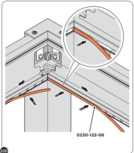
22D MEASURE INSIDE LEG DIMENSIONS AND CUT LED DIFFUSERS (x6) 0230-122-02 TO LENGTH. PUSH AND CLICK INTO THE CHANNELS.
