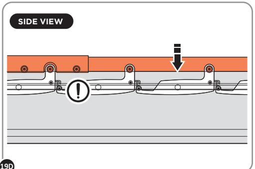
TO ENSURE THE LOUVERS ARE FULLY CLOSED, APPLY A SMALL AMOUNT OF DOWNWARDS PRESSURE BEFORE TIGHTENING UP ALL THE FIXINGS.
