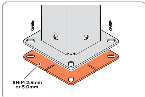
IF THE FOUNDATIONS ARE UNEVEN, SHIM(S) CAN BE ADDED UNDER EACH FOOT AS REQUIRED.
