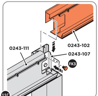
**11C** LOCATE BEAM BRACKET 0243-107. FIT TO SLOTTED HORIZONTAL BEAM. SECURE BOTH BEAMS TO FIXING PLATE 0230-149.
