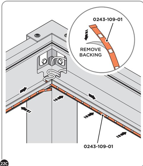
22C LOCATION LED STRIP 0243-109-01, PEEL-OFF PROTECTIVE ADHESIVE BACKING AND ADHERE LED LIGHTS TO BEAM AS SHOWN ABOVE. THE LED STRIP FITS IN THE GROVE ALL ROUND THE FOUR SIDES.
