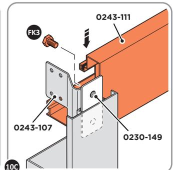
10C LOCATE BEAM BRACKET 0243-107. FIT TO HORIZONTAL BEAM AND SECURE TO LOWER PART OF FIXING PLATE 0230-149.
