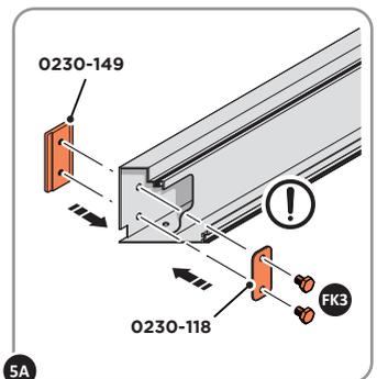
SECURE FIXING PLATES 0230-149 & 0230-118 TO HORIZONTAL BEAMS.
