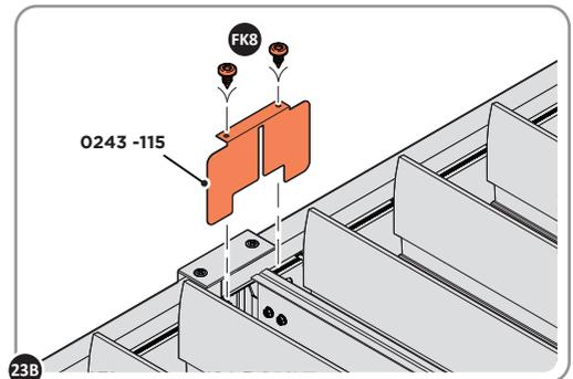
23B LOCATE CENTRE COVER PLATE 0243-115 AND SECURE TO HORIZONTAL BEAM USING SELF TAPPING SCREWS (FK8).
