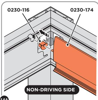
LOCATE AND SECURE LOUVER BEARING 0230-116 ONTO LOUVER 0230-174, SECURE TO BEAM 0243-110 ON NON-DRIVE SIDE.
