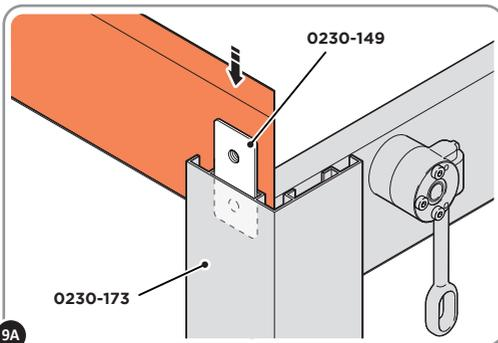
9A ENSURE FIXING PLATE 0230-149, SLOTS INTO TOP OF THE PERGOLA LEG AT BOTH LOCATIONS, AS SHOWN ABOVE.
