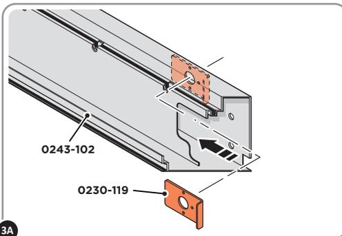
**3A** LOCATE FIXING PLATE 0230-119 INSIDE SLOTTED HORIZONTAL BEAM 0243-102, ENSURING FIXING HOLES ARE ALIGNED.
