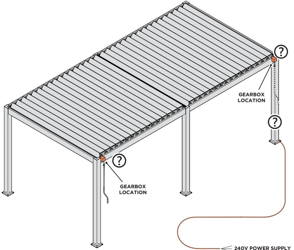
**NOTE:** POWER SUPPLY CAN BE INSTALLED TO ANY OF THE FOUR CORNER LEGS.
