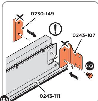
10A LOCATE BEAM BRACKET 0243-107. FIT TO HORIZONTAL BEAM AND SECURE TO LOWER PART OF FIXING PLATE 0230-149.
