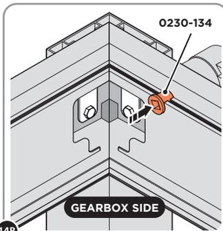
LOCATE AND SECURE DRIVING BUSH 0230-134 TO BEAM 0243-101, AS SHOWN ABOVE.
