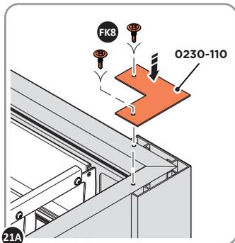
LOCATE CORNER POST CAPS 0230-110 AND SECURE TO PERGOLA LEGS USING (X2) ECO FIX SCREWS (FK8).
