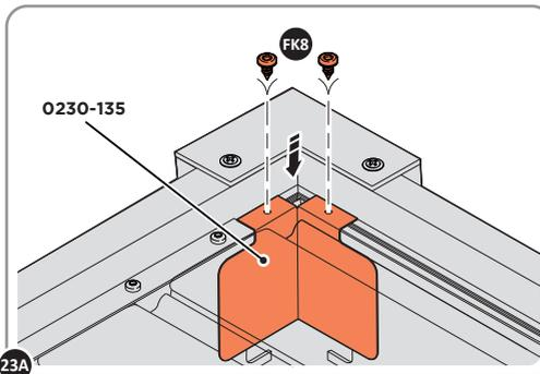
23A LOCATE CORNER COVER PLATE 0230-135 AND SECURE TO HORIZONTAL BEAM USING SELF TAPPING SCREWS (FK8).
