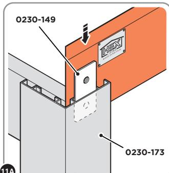
**11A** ENSURE FIXING PLATE 0230-149, SLOTS INTO TOP OF THE PERGOLA LEG AT BOTH LOCATIONS, AS SHOWN ABOVE.
