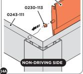
LOCATE AND SECURE LOUVER BEARING 0230-113 ONTO LOUVER 0230-174, SECURE TO BEAM 0243-111 ON NON-DRIVE SIDE.
