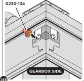
LOCATE AND SECURE DRIVING BUSH 0230-134 TO BEAM 0243-102, AS SHOWN ABOVE.
