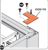
LOCATE CORNER POST CAPS 0230-110 AND SECURE TO PERGOLA LEGS USING (X2) ECO FIX SCREWS (FK8).
