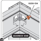
LOCATE AND SECURE DRIVING BUSH 0230-134 TO BEAM 0243-101, AS SHOWN ABOVE.
