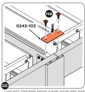
LOCATE CENTRE POST CAPS 0243-103 AND SECURE TO PERGOLA LEG USING ECO FIX SCREWS (FK8).
