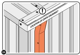
ALIGN DRAINPIPE 0252-18 WITH OPEN GROMMET WITHIN ROOF GUTTER. IMPORTANT: DRAINPIPE BRACKET IS LOCATED WITHIN SIDE PANEL RECESS.
