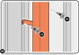
SECURE DRAINPIPE AT x6 LOCATIONS INDICATED USING TYPICAL FIXING METHOD.
