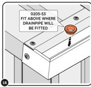
LOCATE AN OPEN GROMMET INTO THE ROOF GUTTER ABOVE WHERE THE DRAINPIPE WILL BE LOCATED.
