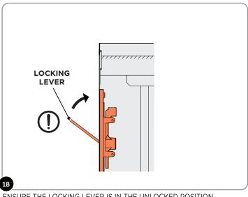
ENSURE THE LOCKING LEVER IS IN THE UNLOCKED POSITION, AS SHOWN ABOVE.
