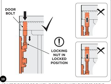
ADJUST THE DOOR BOLT UNTIL IT SITS FLUSH WITH THE EDGE OF THE DOOR. SECURE INTO POSITION WITH THE LOCKING NUT.
