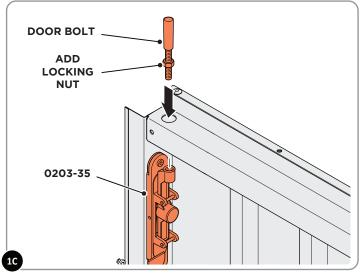
THREAD THE LOCKING NUT ONTO THE DOOR BOLT AND INSERT THROUGH THE HOLE IN THE DOOR AND SCREW INTO THE BOLT BODY 0203-35.
