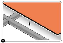
FIRST SLOT FLOOR PANELS INTO THE BACK HALF OF FLOOR FRAME. IMPORTANT: THESE FLOOR PANELS DO NOT HAVE A CUT-OUT.
