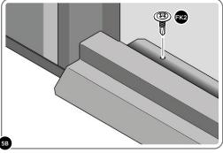
SECURE DOOR STRIP ONTO FLOOR PANELS AT X6 LOCATIONS INDICATED.
