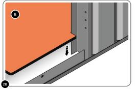
SLOT LEFT-HAND FLOOR PANEL INTO THE FRONT HALF OF FLOOR FRAME. SLOT RIGHT-HAND FLOOR PANEL INTO THE FRONT HALF OF FLOOR FRAME.
